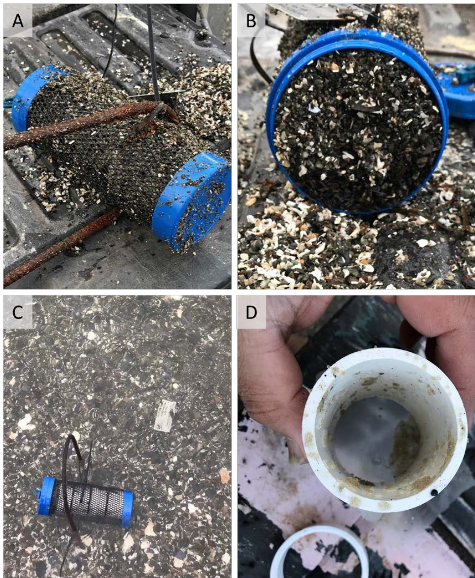
Figure 12: Outer cages allowed movement of sand and shells (A, B, C), while inner embryo chambers remained clear of debris (D).
